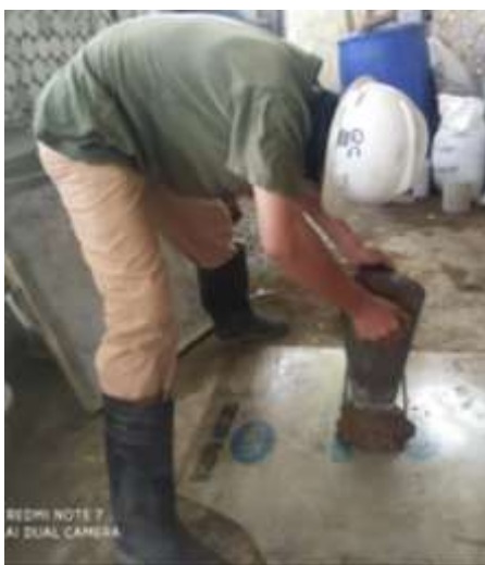
Figure 1 Slump test on fresh concrete.
